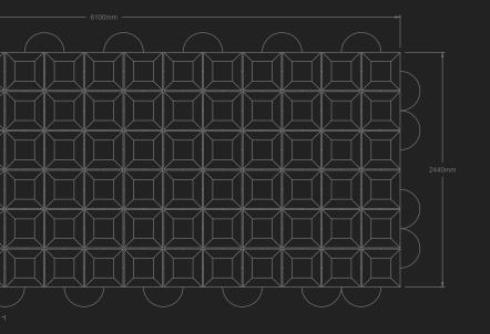
Designed as a marine solution for semi and submerged hard armored applications such as cable, pipeline protection, & outfall scour protection. With a centered ligature structure and a trapezoidal base to each block, the system is designed to be extremely flexible in both upward and downward directions. CC60 is an effective alternative to traditional methods such as rock armoring, sand and grout bags, structural concrete, and other hard armoring systems.
